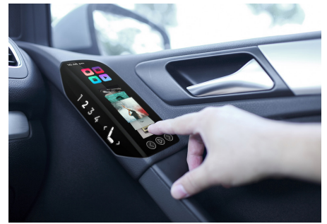
Figure 1 - Flexible display concepts that match the dimensionality of the A-pillar (top) and door frame (bottom) enable seamless, space-saving integration. 2 (Source: Flexenable)
