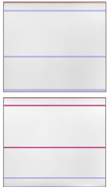
Figure 6 - Horizontal Line Defects analysis performed by a 2MP imaging system (top) versus an 8MP imaging system (bottom). Horizontal lines are noticeably higher contrast using the 8MP imaging system.
