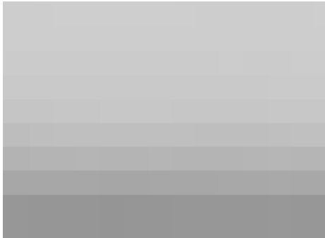
Figure 4 - Close-up of a measurement image showing dark areas on the bottom edge of the display, which are visual effects caused by the horizontal display curvature.
