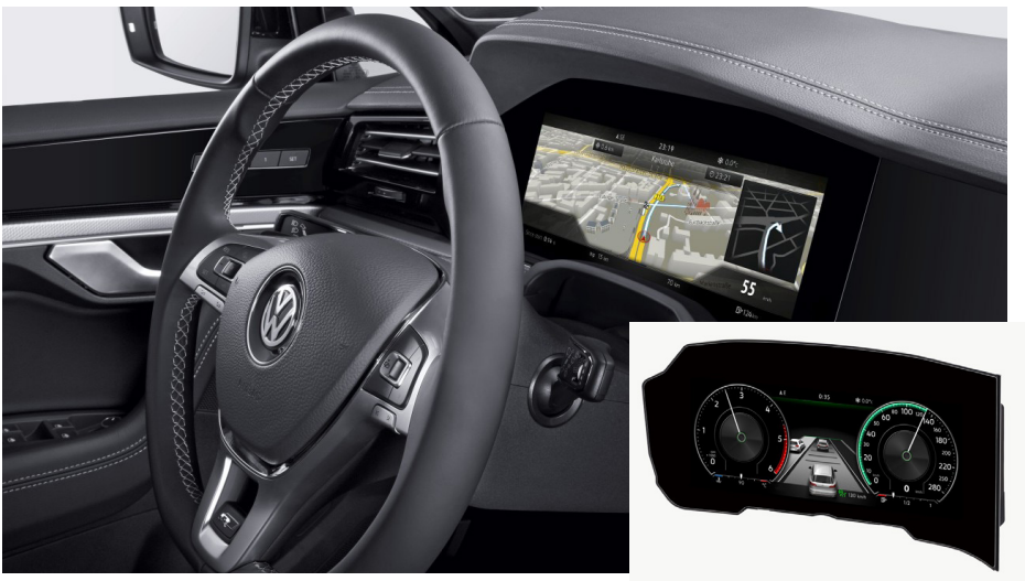
Figure 2 - A curved instrument panel display by Bosch with 1500R (1,500 mm horizontal radius of curvature) at 12.3-inch diagonal size, manufactured for the Volkswagen Touareg, shown inside (left) and outside of the vehicle (right). 3 (Source: Bosch, 2018)
