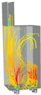
Flue gas flow pattern in the radiant section, path lines colored by temperature.
