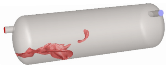
Iso-surface of liquid volume fraction shows that the separated liquid layer is being re-entrained to the vapor phase.
