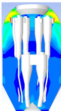
Velocity distribution across the FCCU
