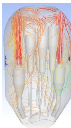
Path lines colored by temperature showing evaporation of the quench spray
