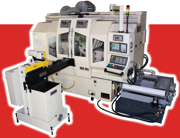
▲ TGS-CL-6020 CNC centerless grinder with elevator hopper, loading conveyor and post-process gage for throughfeed pin grinding
