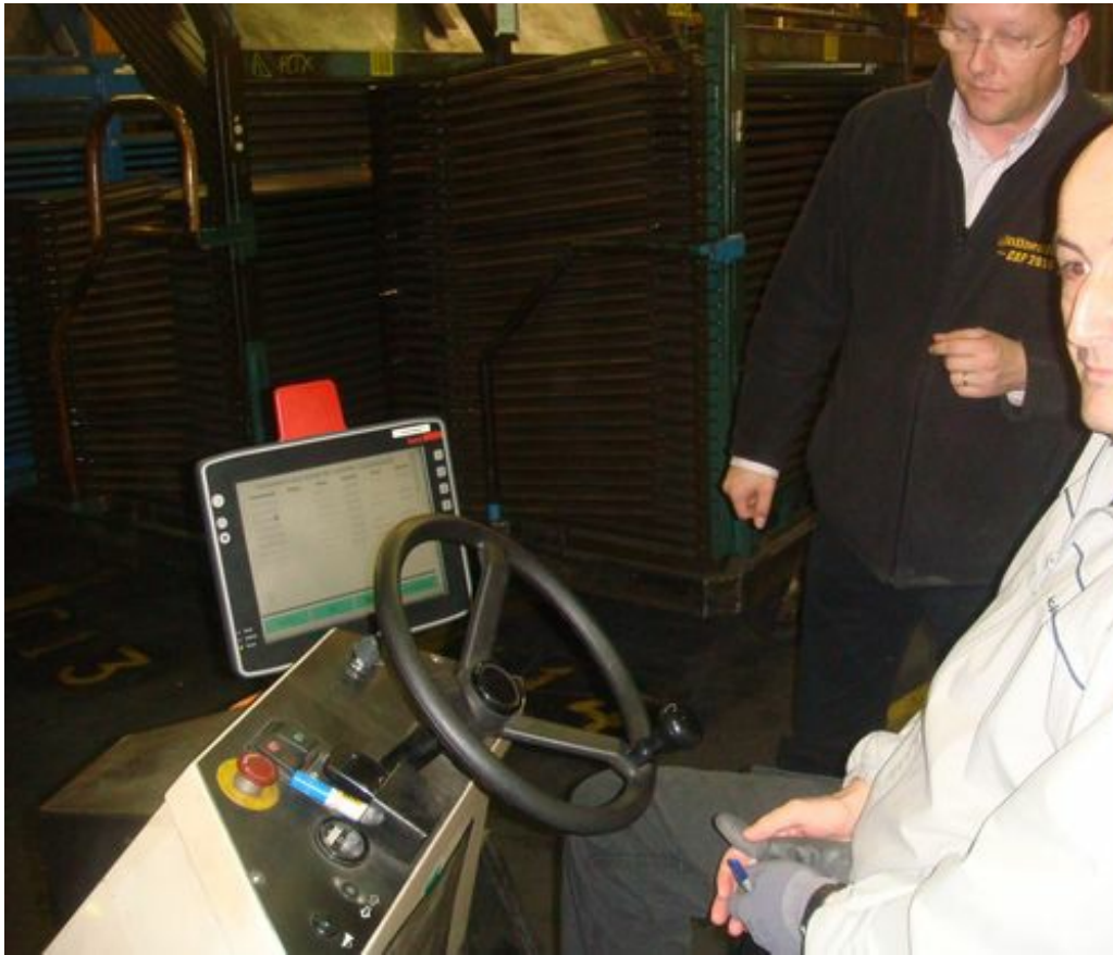
A tugger's driver can view his vehicle's computer screen to identify the locations of carriers he needs to move.
