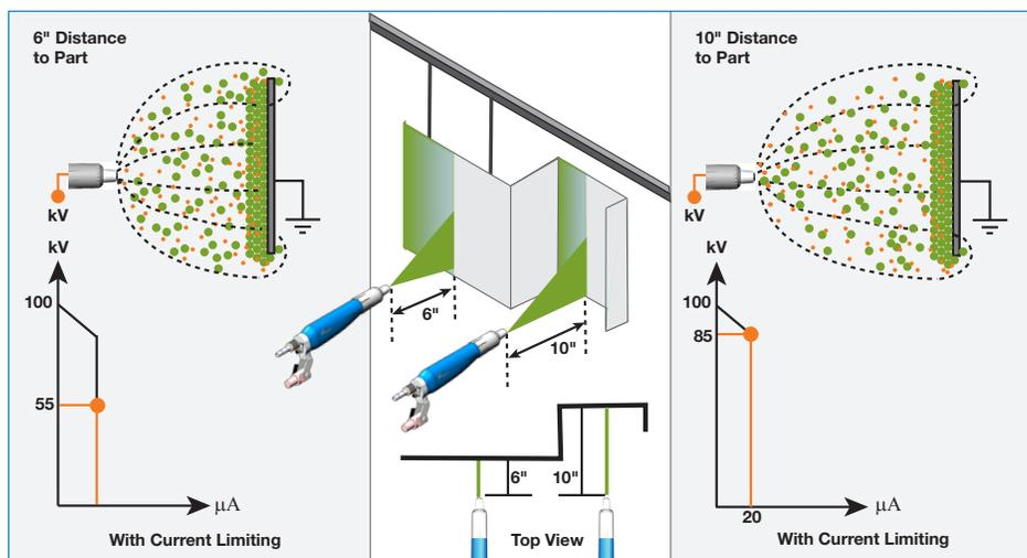
ions will flow through a narrower channel causing a higher current density per unit of the part’s surface; and 2) a closer gun-to-part distance will result in a higher current level which, following our analogy, would be equal to increasing the volume of water flowing through the hose. Therefore, at a 3-inch gun-to-part distance, conditions are such that even a gun current which is optimal for 6 inches, is enough to cause rapid development of back ionization and lower transfer efficiency.
