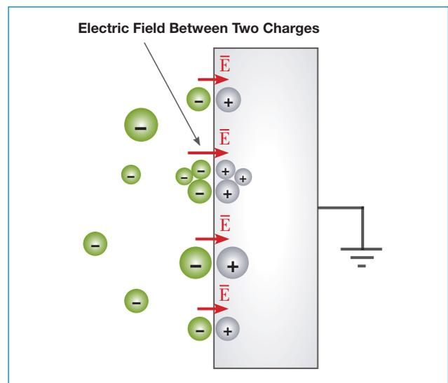
induction process (since there is no direct contact of powder particles with the metal surface). Lower charges of smaller particles may not be sufficient to create an attraction force strong enough to retain the particles on top of the already deposited powder coating layer.
