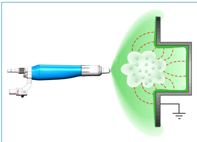
coated regardless of how long powder is sprayed. In some cases, this happens because of the geometry of the recess and problems with air turbulence, but often times it is due to back ionization.
