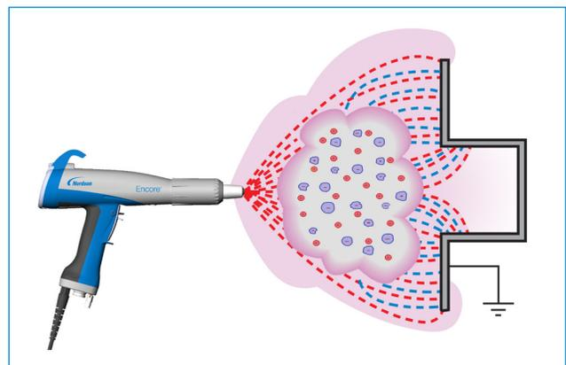
electric field towards the edges of Faraday cage. Second, free ions generated by the corona discharge will follow field lines toward the edges, quickly saturate the existing coating with extra charge, and lead to very rapid development of back ionization.
