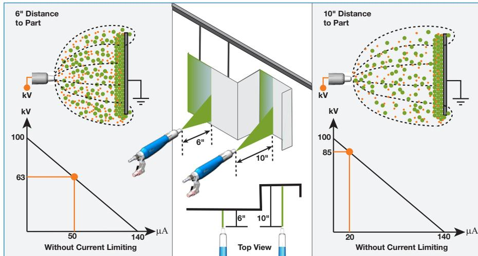
Results of experiments show that for a broad range of gun-to-part distances there is some current level that provides for maximum transfer efficiency. Therefore, if we had a tool that would allow us to automatically maintain gun current at this optimum level (regardless of the gun-to-part distance), we would optimize overall efficiency of the powder coating process. This tool is automatic current control (ACC).
