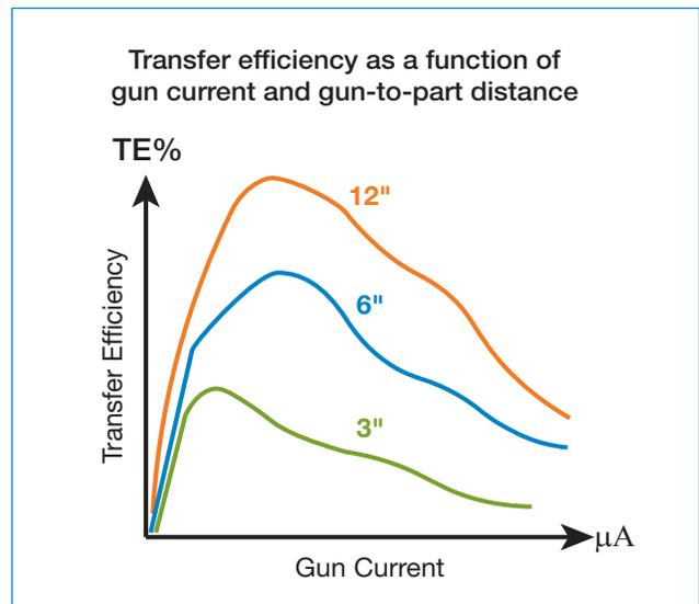
distance of 3 inches will be significantly greater than the number of ions flowing to the part at a gun-to-part distance of 10 inches.
