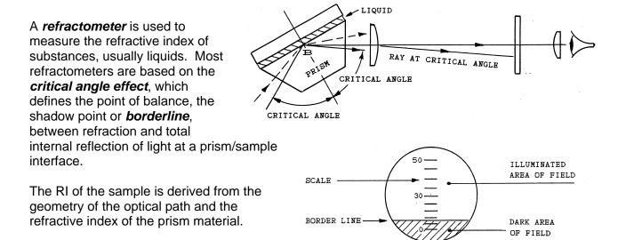
Modern *digital automatic refractometers* use a light sensitive integrated circuit (self-scanned array) to detect the exact position of the borderline. Bellingham+Stanley instruments also incorporate special software for interpreting 'fuzzy' borderlines that many products tend to produce. In this way, there is no subjective human judgement needed in taking a reading - a major advantage of an automatic instrument.
