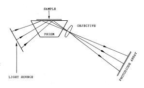
When the composition of a substance changes, so does its RI. Thus a measure of RI can yield information about the composition of a substance. For example, when a substance is dissolved in a liquid the RI increases. Thus a measure of the RI of a sugar solution in water can be used to determine the *solution concentration*.
