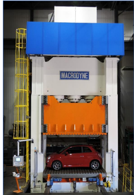
Macrodyne 2000-400 ton single-acting Deep Draw press with hydraulic cushion & rolling
