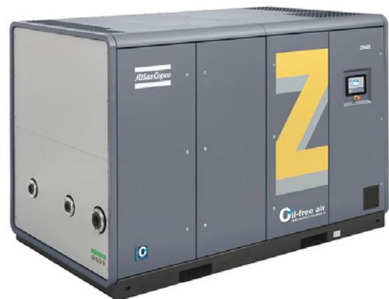
Depending on the design, oil may be used to cool other moving components, but it will never contact the actual compressed gas. Without a fluid medium to cool and seal, oil-free air temperatures run hotter and typically employ a larger aftercooler.
