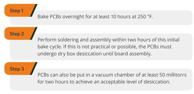
Desiccation is the most crucial step before soldering, particularly with flexible and rigid-flex PCBs. Not following these moisture removal guidelines could lead to post-assembly defects.
